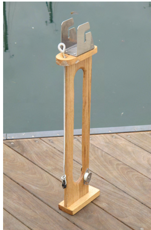
A mast support post must be strong enough to carry the mast's weight and downward pressure.
