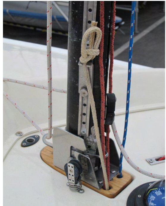
When the standing rigging is secured the halyards, vang and cummingham may be lead below or secured at the mast base.
